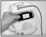
4. Put the battery pack into the unit, making sure to orient it as shown.
