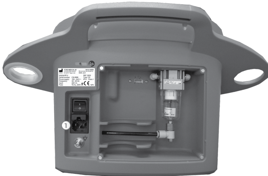
Fig. 2 - 3 Connecting power supply cables
