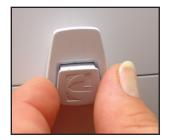
Insert the Patient Interrupt Switch Hook Cover to cover the hook screw hole.
