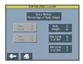
For Percentage of Body Weight, Press the Body Weight button and enter the body weight of the patient. Press the Max. Level % of BW button to enter the percentage of the patient's body weight to be the maximum traction tension level. Press the Min. Level % of BW button to enter the percentage of the patient's body weight to be the minimum traction tension level.
