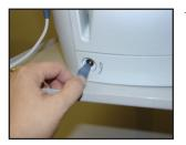
1. Attach the Patient Interrupt Switch by inserting the male end of the cable into the Patient Interrupt Switch Receptacle located on the front of the unit.
