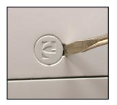
A screw hole cap with the Chattanooga logo is located on both sides of the traction unit.
